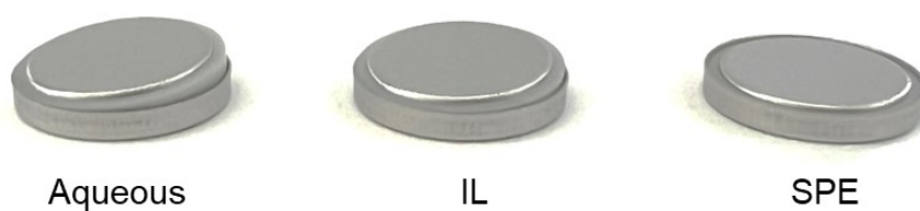
Figure S12. Optical pictures of the coin cells with the aqueous electrolyte, IL electrolyte, and SPE after cycling at 90 \text{ }^\circ\text{C} . The cells with the aqueous and IL electrolyte display evident expansion and damage, whereas the cell with the SPE shows remarkable stability, remaining unchanged throughout the cycling process.
