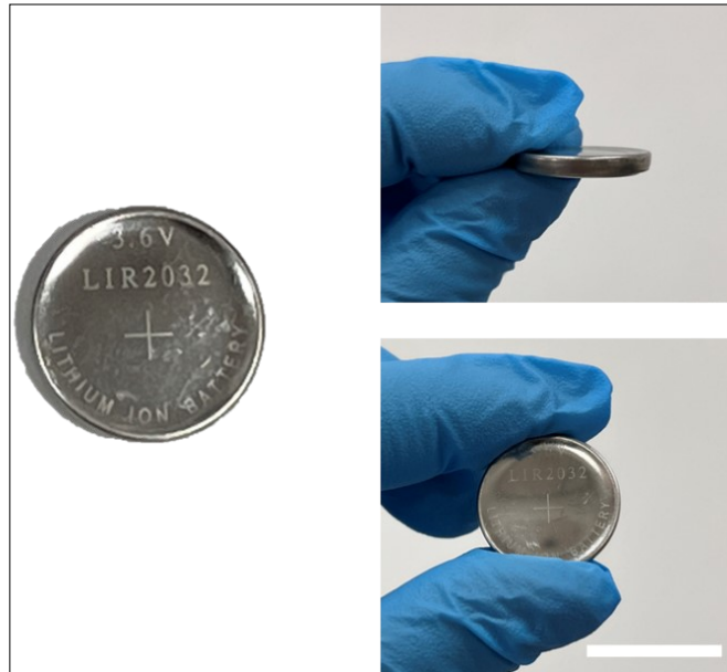
Supplementary Fig. S18. Coin cells with the size of \phi=15.6 mm assembled from two stainless steel tabs holding Zn-TFMS-PC/TEP electrolyte.
