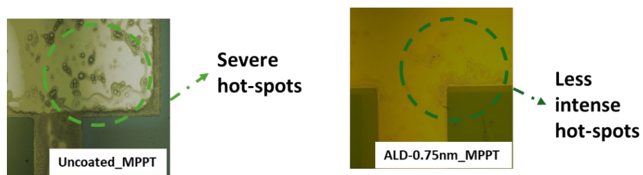
Figure S17. Optical images of the uncoated and ALD-0.75nm devices from the glass side illumination after the MPPT test.
