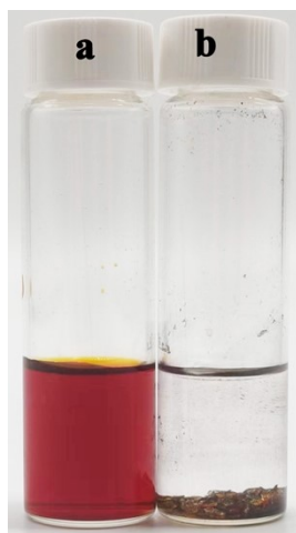
Fig. S3 Images of a) the polyiodide solution, and b) the polyiodide solution with TBAI. Upon the addition of TBAI to the polyiodide solution, the color of the polyiodide solution transitioned from brownish-red to colorless, indicating the robust adsorption of TBAI on polyiodide ions.
