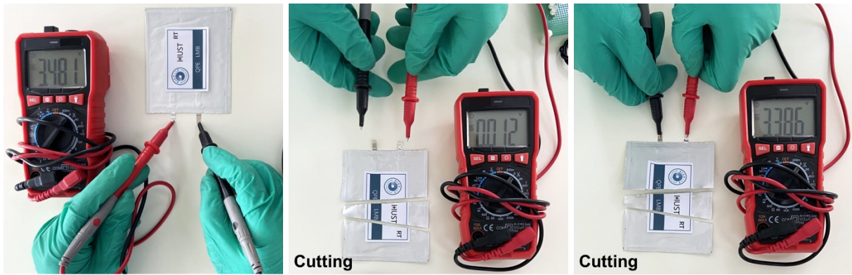
Figure S41 Optical photographs of the voltage test by subjecting a pouch cell to cutting.
