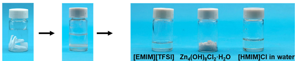
Fig. S35 Photos of the recyclability of HZLE-1. [HMIM]Cl was dissolved in water, while [EMIM][TFSI] was insoluble in water and Zn_4(OH)_8Cl_2 \cdot H_2O was precipitated in water. Thus, [EMIM][TFSI] was separated by liquid-liquid phase separation and the Zn_4(OH)_8Cl_2 \cdot H_2O and [HMIM]Cl were obtained by filtration.
