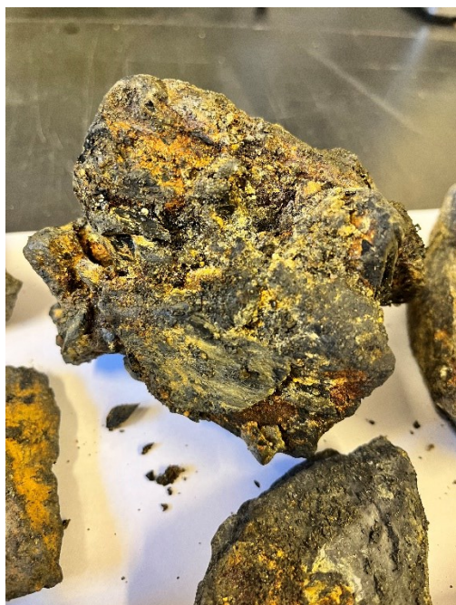
Fig S5. Representative pictures of soil core sampling (top) and alum shale waste rocks (bottom) at the Taraldrud site. For soil sampling: a plastic corer tube was vertically inserted into the soil or sediment followed by careful excavation in order to retrieve an intact core. During the sampling at the P and MZ site locations, orange-brown color was observed on the top layers, suggesting the presence of iron-rich solid phases. Alum shale sampling was carried out by NGI in 2021. 3
