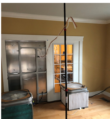
Figure S3. WSOC sampling inlet locations. Room air was drawn to the MC ( WSOC_g ) and PILS ( WSOC_p ) through the Teflon tube and copper tube, respectively.
