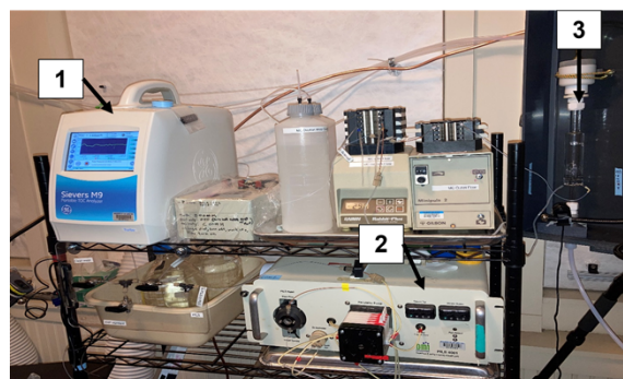
Figure S2. Instruments for WSOC_g and WSOC_p on NZERTF porch. 1. Total organic carbon analyzer (TOC) 2. Particle-into-liquid sampler (PILS) 3. Mist Chamber (MC).
