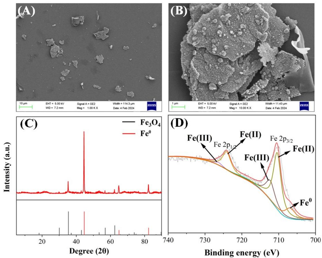
Fig. S1 SEM images (A-B), XRD (C), and XPS (D) analyses of the Fe<sup>0</sup> nanoplates.
