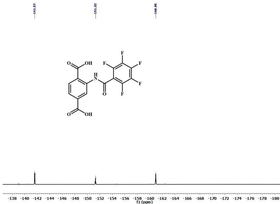
Fig. S3. 19 F NMR spectrum of 2-(perfluorobenzamido)terephthalic acid linker in DMSO-d 6 .
