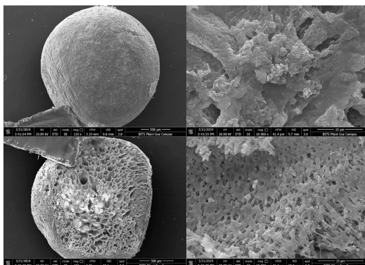
Figure S13: SEM images of the full and cross-section TP beads reused after 30 cycles of photocatalysis, TP = 1% TiO 2 with PVDF having 0.7 % PVP.
