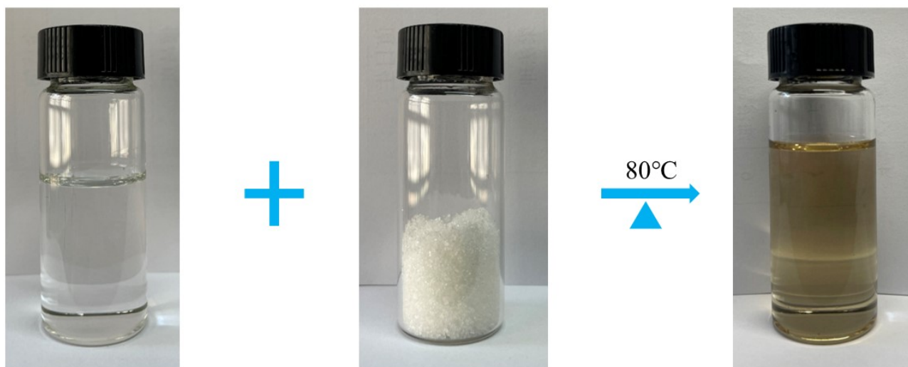
Fig. S1 Flow chart for synthesis of \text{AlCl}_3 \cdot 6\text{H}_2\text{O} : Glycerol (1:8 mol/mol) DESs.
