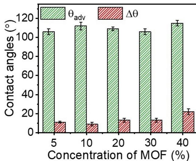
**Figure S3.** Effect of filler concentration on wettability of the WPU-MOF coating. Error bars represent standard deviation from at least four different measurements at different locations of the coating. WPU-MOF nanocomposites with varying filler concentrations were prepared to determine optimal nanoparticle concentration with best possible liquid repellency.
