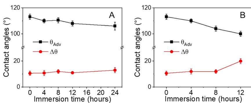
**Figure S12.** Chemical stability of WPU-MOF coating. Variation of  $\theta_{Adv}$  and  $\Delta\theta$  in (A) acid (pH~1-2), and (B) alkali (pH~12-13) solution over a period of 24 hours.
