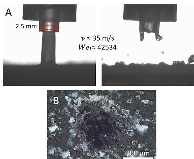
**Figure S11.** (A) Snapshots of 2.5 mm water jet impacting on WPU-SiO<sub>2</sub> coating vertically with a speed of 35 m/s. (B) 3D-microscope image of WPU-SiO<sub>2</sub> coatings on glass after repeated jet impacts (3 times) at 35 m/s.
