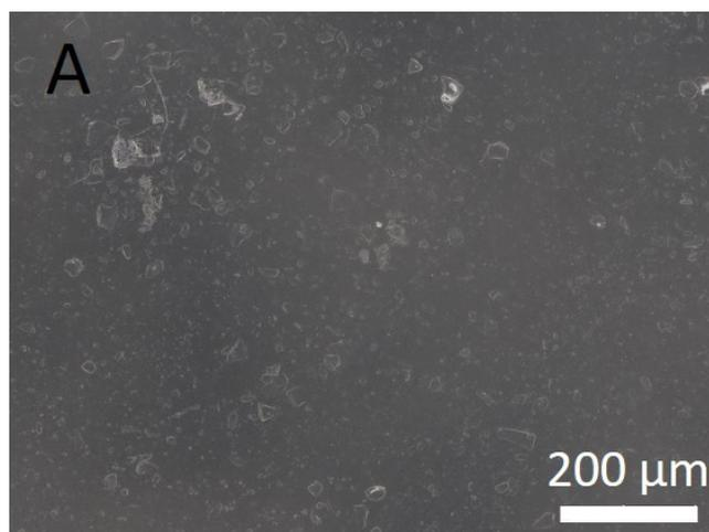
**Figure S10.** 3D-microscope image of WPU-MOF on glass after repeated jet impacts (3 times) at 35 m/s.
