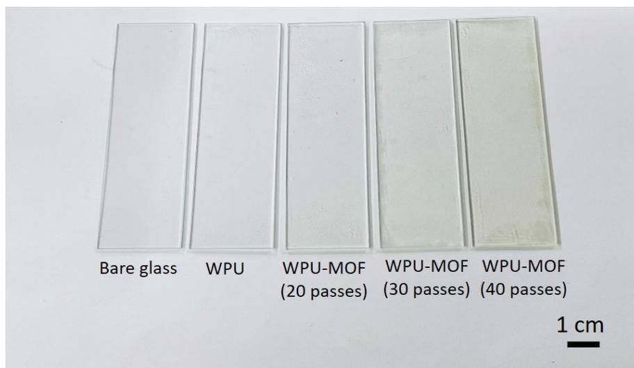
**Figure S6.** Samples showing effect of spray passes on the transparency.
