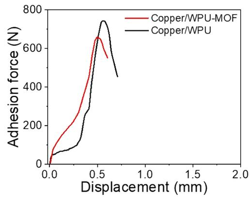
**Figure S7.** Force-displacement curves for adhesion testing of copper lap joints coated with WPU and WPU-MOF nanocomposite.
