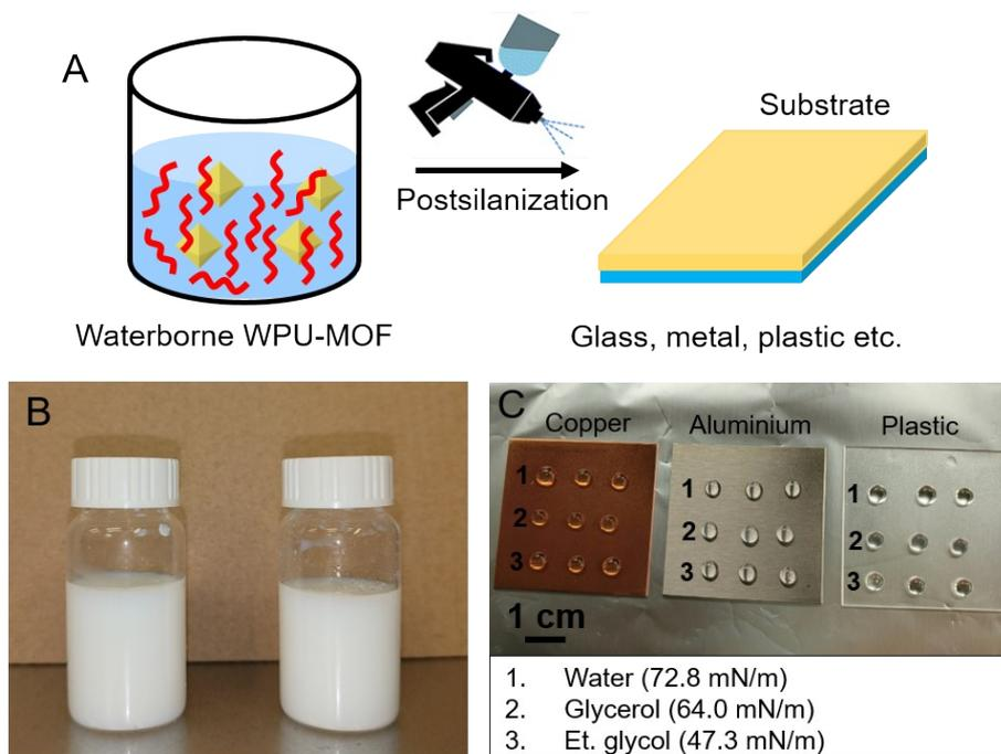
**Figure S5.** (A) Schematic illustration of WPU-MOF coating via spraying. (B) WPU/MOF/water suspension as prepared (left vial) and stored at room temperature for 1 month (right vial). (C) Optical image of WPU-MOF coating on different substrates: copper (50 mm × 50 mm), aluminium (50 mm × 50 mm), and plastic (50 mm × 50 mm). Liquid droplets of different surface tensions are placed on coated surfaces; 1) Water, 2) Glycerol, and 3) Ethylene glycol.
