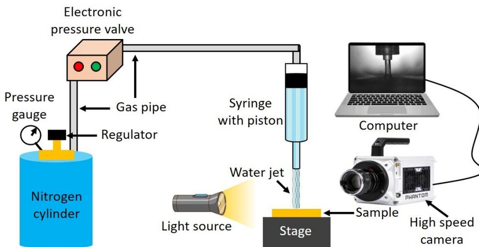
**Figure S9.** Schematic of water jet impact setup.
