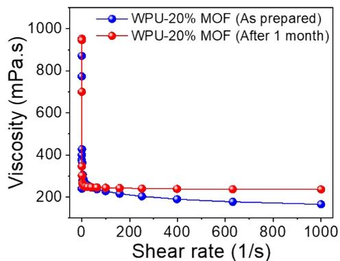
**Figure S4.** Shear viscosity of WPU-MOF coating immediately after preparation and following one month of storage.
