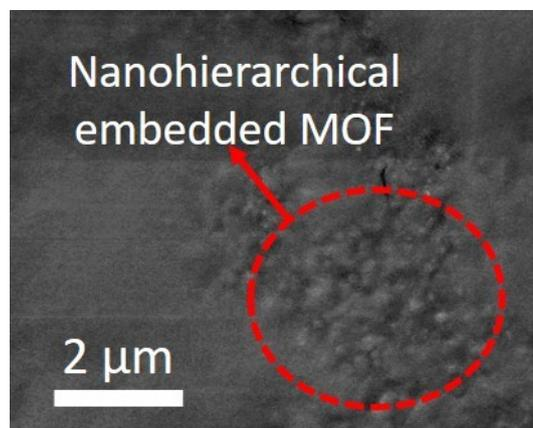
**Figure S8.** SEM image of nanohierarchical MOF embedded into WPU matrix.
