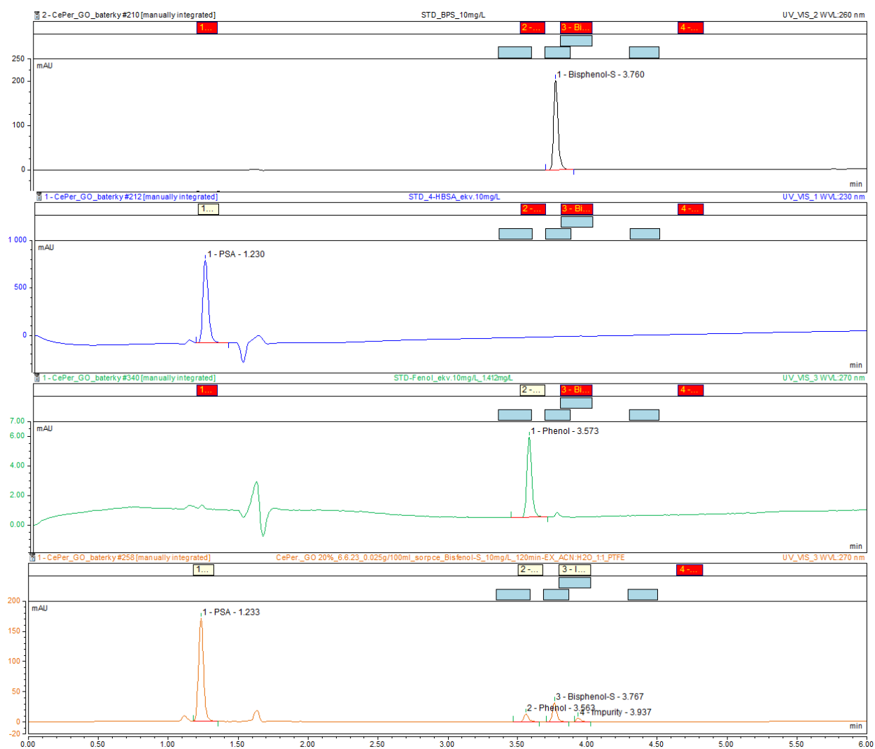
Figure S5. HPLC chromatograms of standards of (top to bottom) BPS, PSA, phenol and the selected chromatogram of BPS reactive adsorption on CeGO20 at time 120 min.
