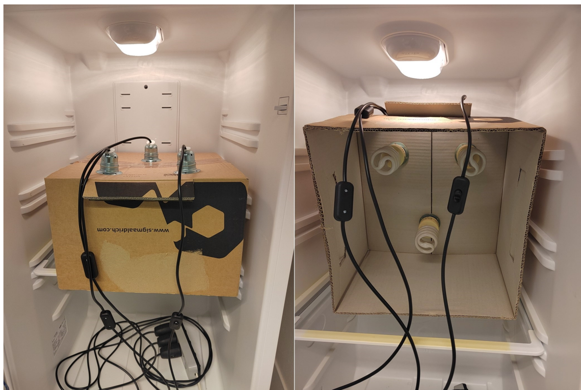
Figure S2. Three UV-B lamps were mounted in a cardboard. Ventilation slits were cut in the box. The box was placed on a shelf in a fridge. The temperature was stable at 22 °C when the three UV-B lamps were on. The samples were placed on the fridge shelf and covered with the box.
