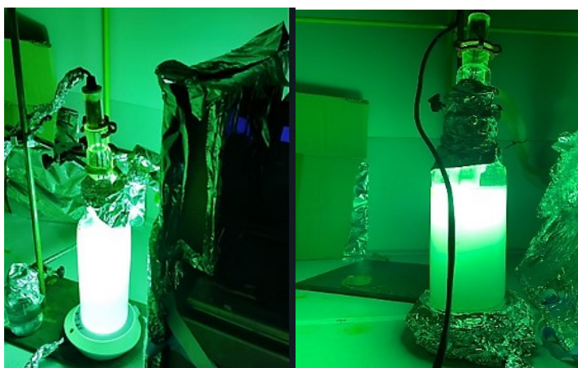
Text S1 Fig. 2: 9.34 kW m -2 at 4 cm medium-pressure mercury lamp (Novalight TQ150) used for the protocol.
