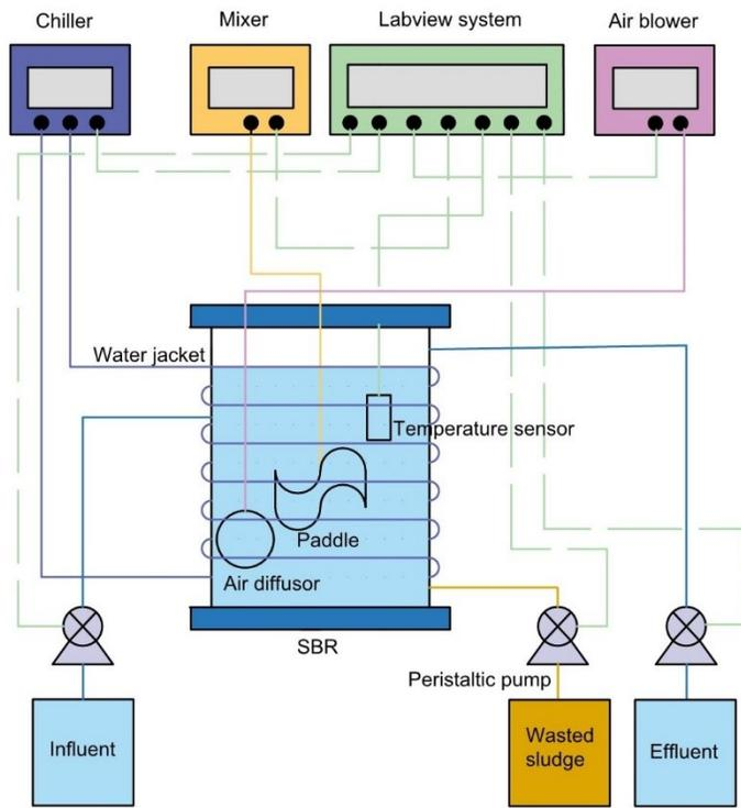
**Fig. S1. Schematic of laboratory-scale SBR.**
