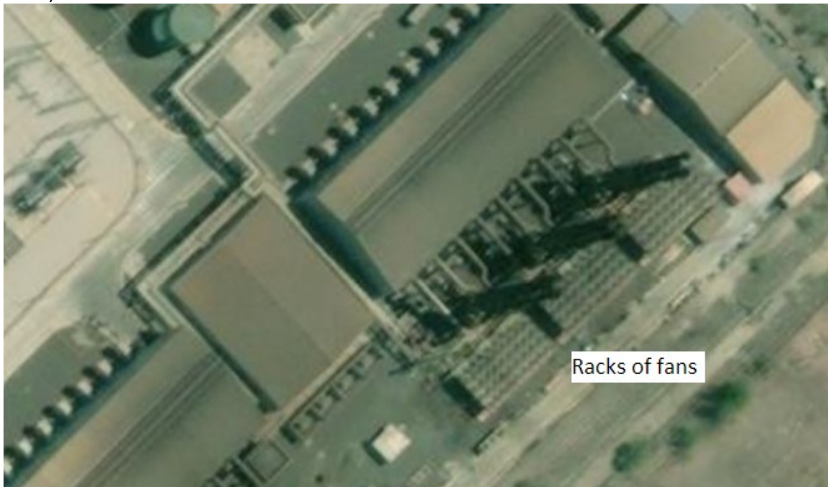
Figure 7a-b. Examples of the infrastructure seen in Satellite Images of Dry Cooling systems.
