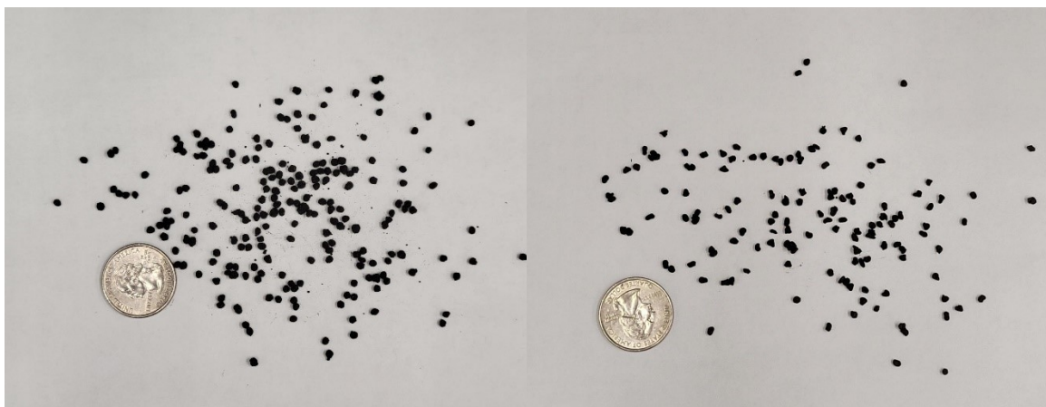
Figure S 1. Calcium alginate beads (made with sodium alginate, PAC, wood flour, Fe-WTR, calcium chloride) [left] and Iron (III) alginate beads (made with sodium alginate, PAC, wood flour, Fe-WTR, Ferric chloride) [right]. Final dried beads (~3mm) decrease in diameter by approximately half from the wet size; coin shown for size reference is a US Quarter.
