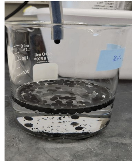
Figure S 5. Bead formation in calcium chloride solution. The wet beads are approximately 6 mm in diameter.
