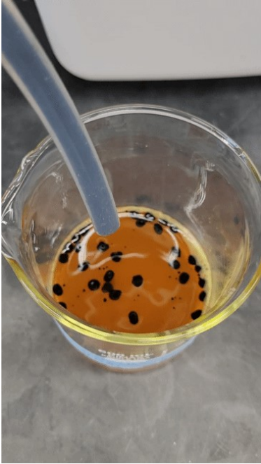
Figure S 8. Making of PAC-wood flour beads with sodium alginate and ferric chloride.
