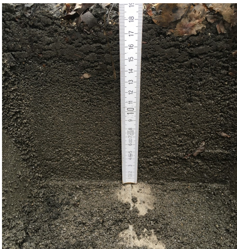
Figure S1: Vertical profile of the filter substratum channel of SCM-D with the sorptive filter media
