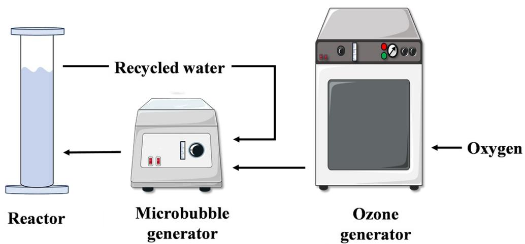
**Fig. S1.** Schematic of experimental setup
