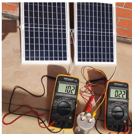
Figure S23 A picture displaying a commercial silicon solar cell-powered \text{Ru}_{0.1}\text{-NiFeOOH/PO}_4^{3-}||\text{Ru}_{0.1}\text{-NiFeOOH/PO}_4^{3-} seawater electrolysis with 1\text{ cm}^2 electrodes operating at 1,020\text{ mA cm}^{-2} under 2.2\text{ V} ( 25\text{ }^\circ\text{C} ).
