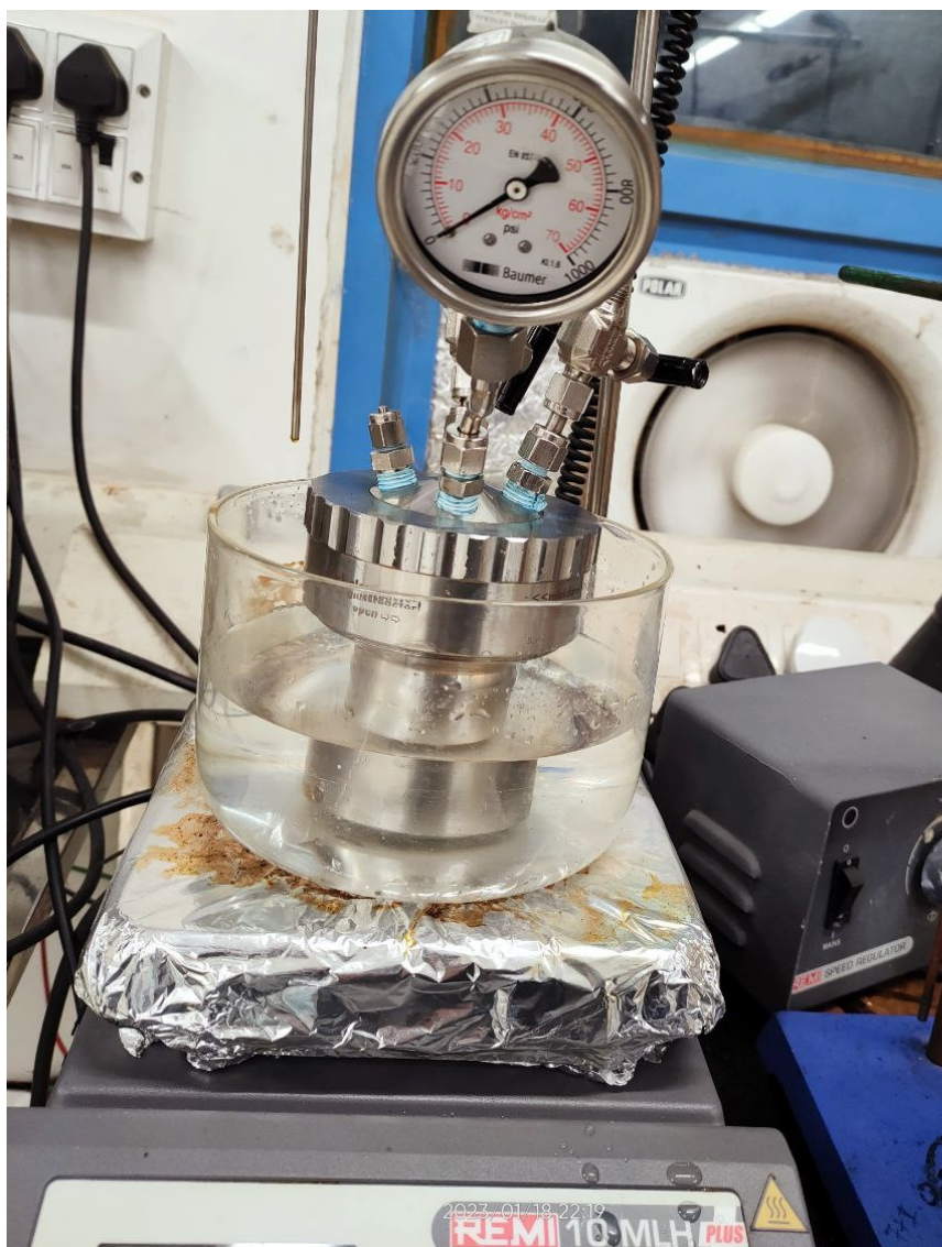
Fig. S2. The digital image of Büchi pressure reactor and reaction setup for the thermal hydrogenolysis of BPE.
