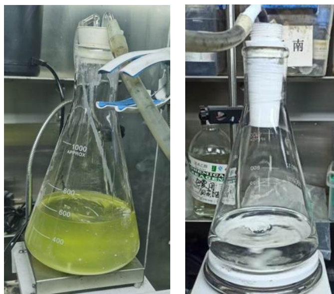
Fig. S4. Color comparison of products of carbothermal reduction (left) and \text{H}_2 reduction (right) dissolved in anhydrous ethanol.
