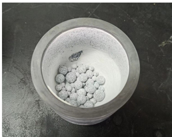
Fig. S3. Photograph of low ball milling efficiency caused by \text{Li}_2\text{SO}_4 sticky wall (ball spinning over material) in dry ball milling.
