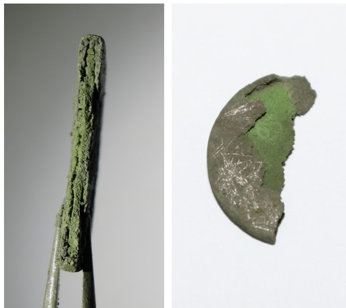
Fig. S2. The cross-section of electrolytic product under constant voltage of 1 V for 6h in LiCl melt.
