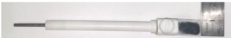
Fig. S1 The photo of the working electrode used in electrochemical experiments.
