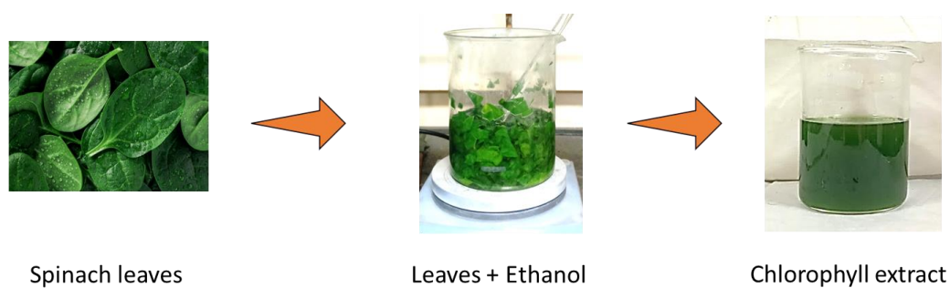
Figure. S29. Schematic diagram for chlorophyll extraction from spinach leaves at temperature of 80-85°C.
