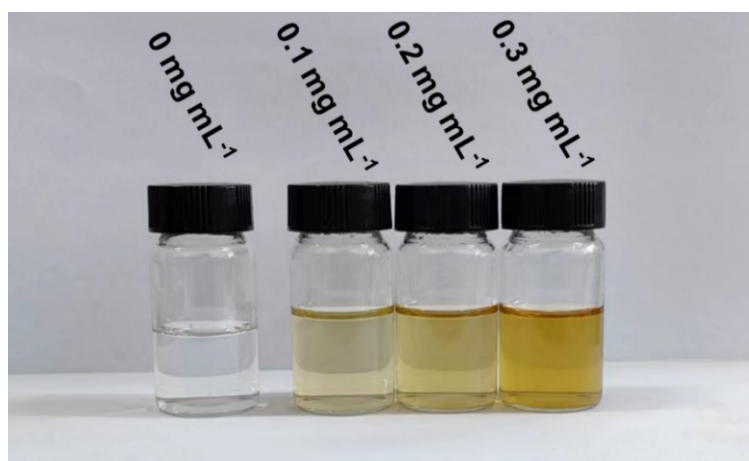
Fig. S2 Optical images of 2 M ZnSO 4 electrolytes at different concentrations of CQDs.
