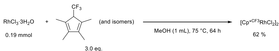
Scheme S1. Preparation of \text{Cp}^*\text{CF}_3\text{H} and [\text{Cp}^*\text{CF}_3\text{RhCl}_2]_2
