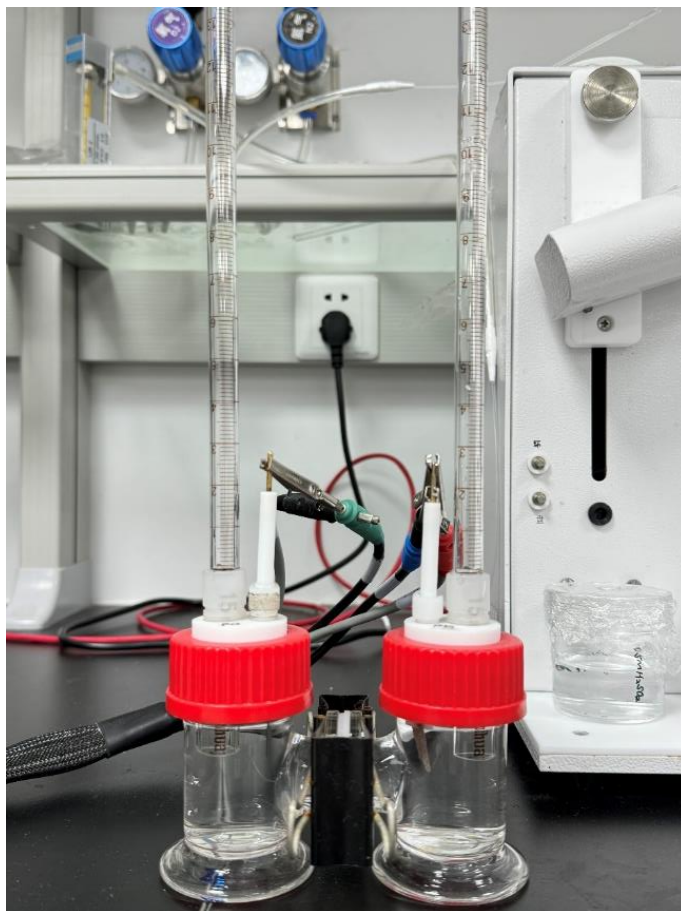
Fig. S28 Schematic diagram of the apparatus for the Faraday efficiency test.
