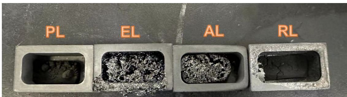
Figure S2 Digital photos of lignin-derived hard carbon materials.
