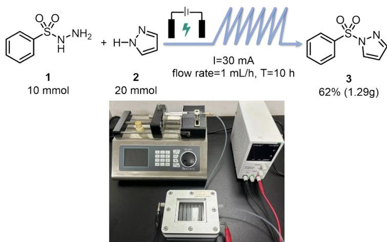
Figure S6. Components of flow chemistry: Micro syringe pump (DK INFUSETEK, SPLab02), DC stabilized power supply (HYELEC, HY3005B), Continuous flow panel (EZONE, PER-10).
