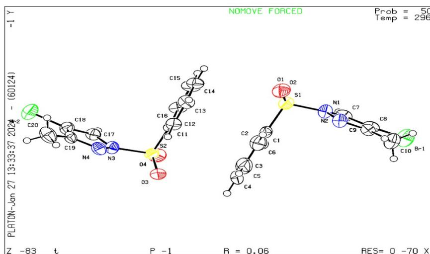
**Figure S8.** ORTEP diagram of compound **23** with ellipsoid shown at the 50% contour percent probability level (CCDC- 2328851)
