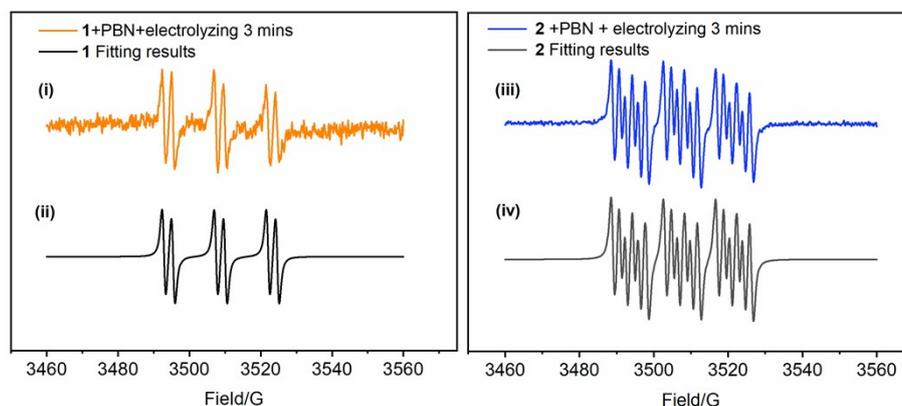
**Figure S3.** EPR experiments: (i) A solution containing PBN, **1**, and CH<sub>3</sub>CN was electrolyzed for 3 mins under N<sub>2</sub> atmosphere, (iii) A solution containing PBN, **2**, and CH<sub>3</sub>CN was electrolyzed for 3 mins under N<sub>2</sub> atmosphere; (ii and iv) Fitting results.
