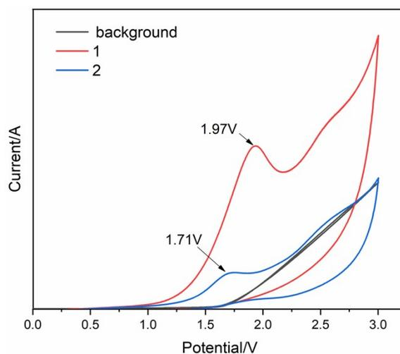
**Figure S4.** The cyclic voltammetry experiment of **1** and **2** in CH<sub>3</sub>CN under air atmosphere.
