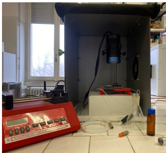
Figure S6. Overall view of the flow set-up employed for this protocol, a box equipped with a fan inside, a syringe-pump that pushed the solution from the coiled tube reservoir to the channel of the reactor where the mixture was irradiated by a 427 nm emission centred KESSIL lamp. The photolyzed solution is recovered in an Erlenmeyer flask.
