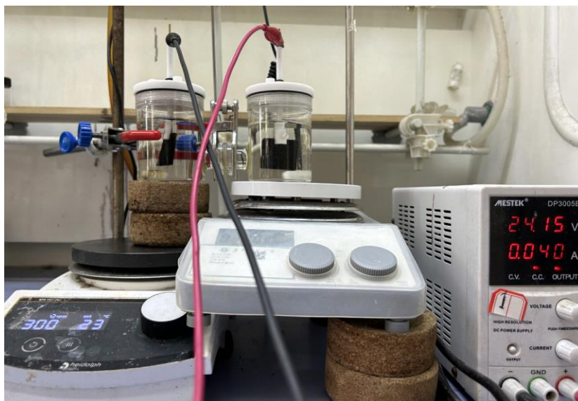
Figure S1 Reaction conditions: cathode: 1 (20 mmol), H 2 O (5.0 equiv), n Bu 4 NClO 4 (0.15 M) in DMF (150 mL); anode: H 2 O (5.0 equiv), n Bu 4 NClO 4 (0.15 M) in DMF (150 mL), graphite felt (GF) as anode and cathode in an H-type divided cell, room temperature, CCE = 40 mA, 49 h, air atmosphere. Yields of isolated products. GF = graphite felt; CCE = constant current electrolysis.
