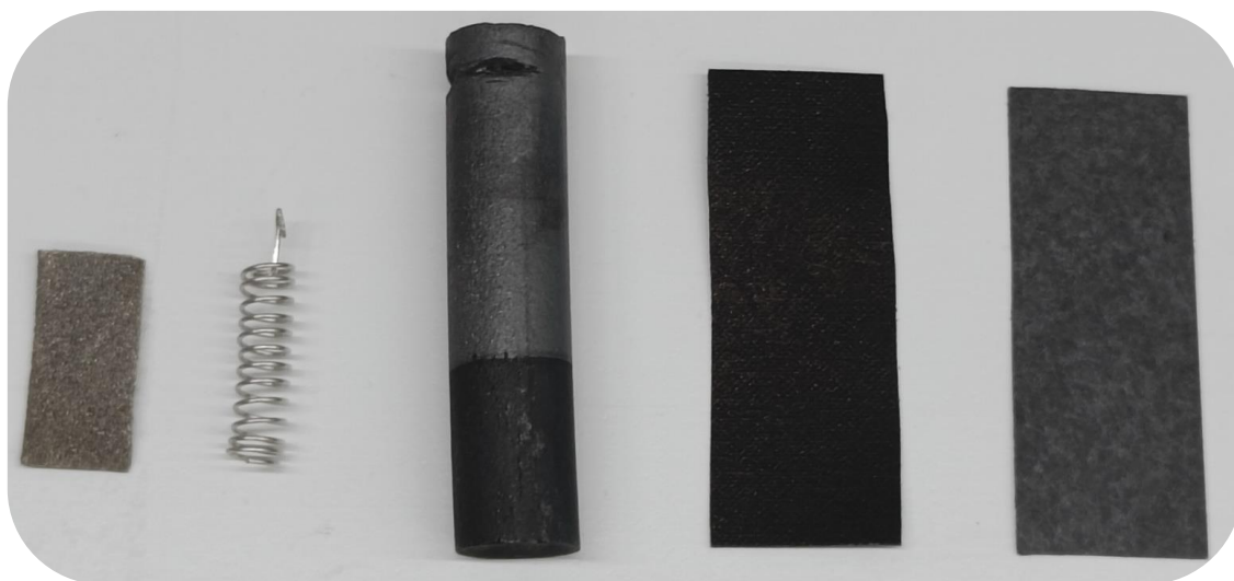
Figure S3. Different counter electrodes employed in the electrochemical hydrogenation of alkenes. From left to right: nickel foam, platinum wire, graphite bar, carbon cloth and carbon paper.
