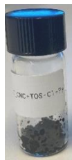
Figure S14: Degradation of cellulose in the attempt to carry out tosylation with the aging process (55°C).
