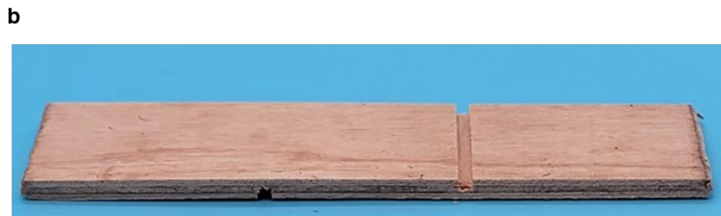
Supplementary Fig. 25 (a) Dimensions of plywood shear strength test samples. (b) Photo of testing sample of plywood.
