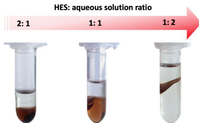
Figure S1. Influence of HES: aqueous solution ratio on blood precipitation.
