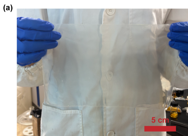
Figure S5. (a) The CPF with a large format exhibits high transparency. (b) The optical transmittance of CPF in the visible light region.
