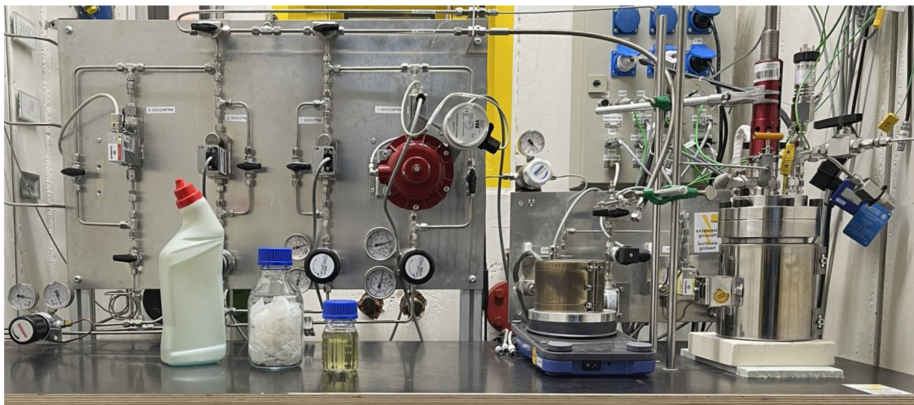
Fig. S12.: Picture of laboratory plant used for carrying out ISOMET reactions in 900 mL.
