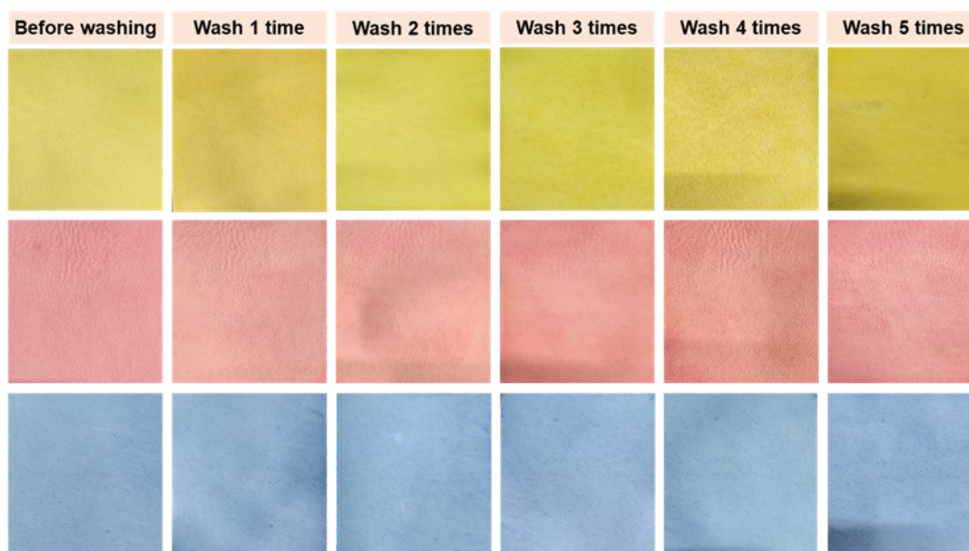
Fig. S10 Color Changes on the surface of AAD-dyed leather after 1 to 5 wash cycles.
