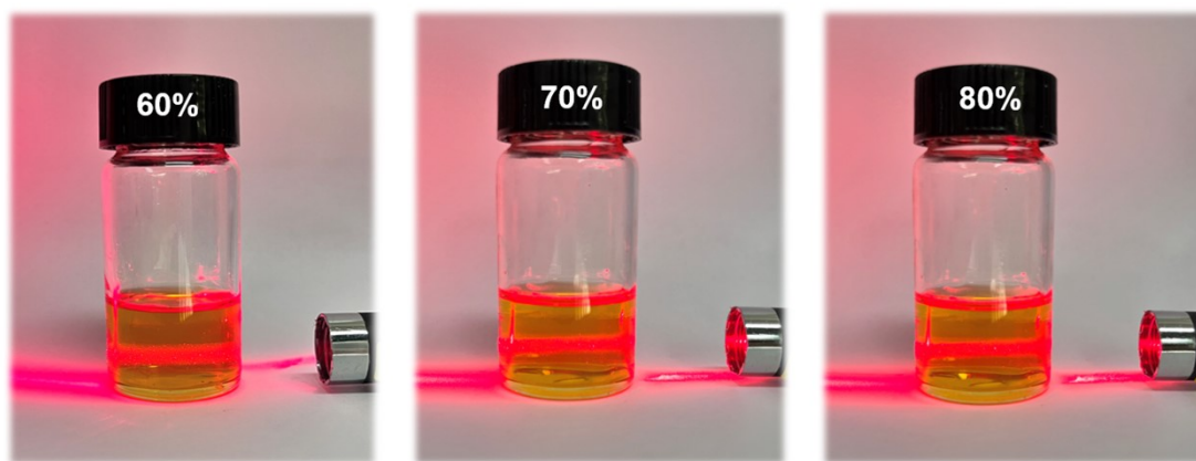
Fig. S7. Tyndall scattering effect of DOPO-TBD:SA polyester at 60%-80% high solid content in water
