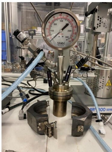
Figure S2: Commercial 30 mL Parr autoclave used for the HCl-catalyzed O-demethylation.
