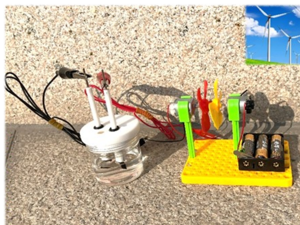
Figure S26. Diagram of urea-assisted water splitting driven by wind power.
