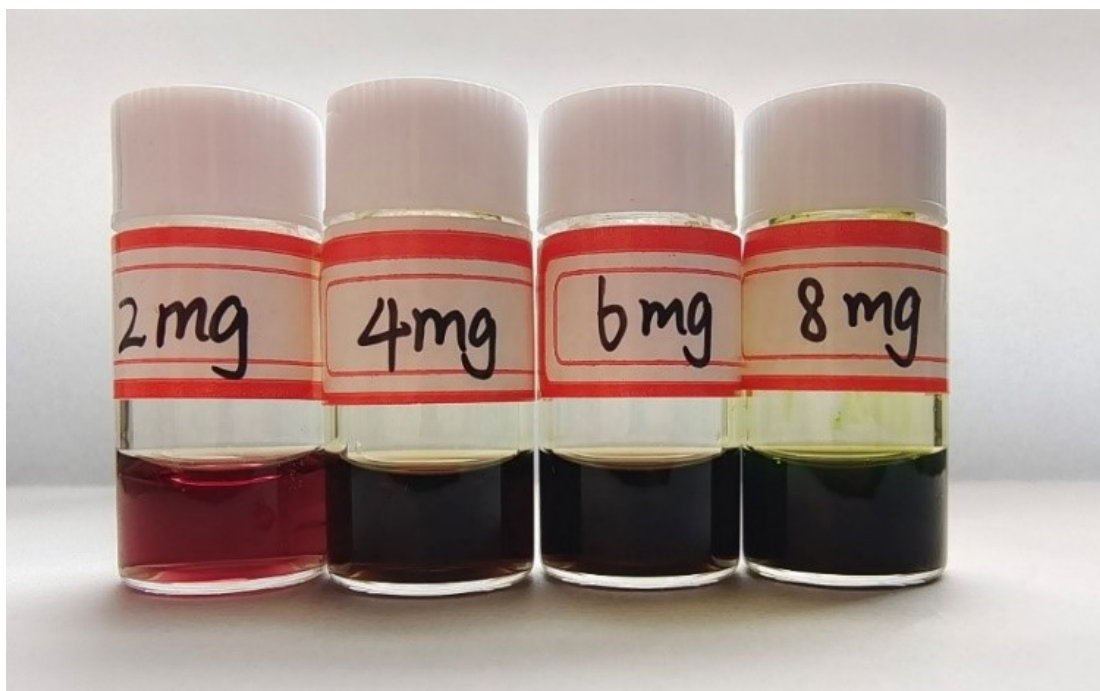
Fig. S3. Digital photos of 2 M \text{ZnSO}_4 + TPPS-2, TPPS-4, TPPS-6 and TPPS-8, respectively.
