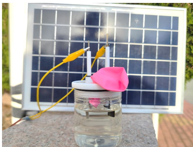
Fig. S29 The photo shows the initial state of the balloon in 1 M KOH + 0.33 M urea.
