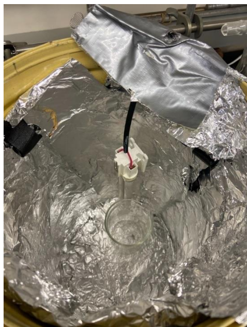
Figure S2. Photo of the photoreactor containing the Rexim G23 UV-A (9W) lamp.
