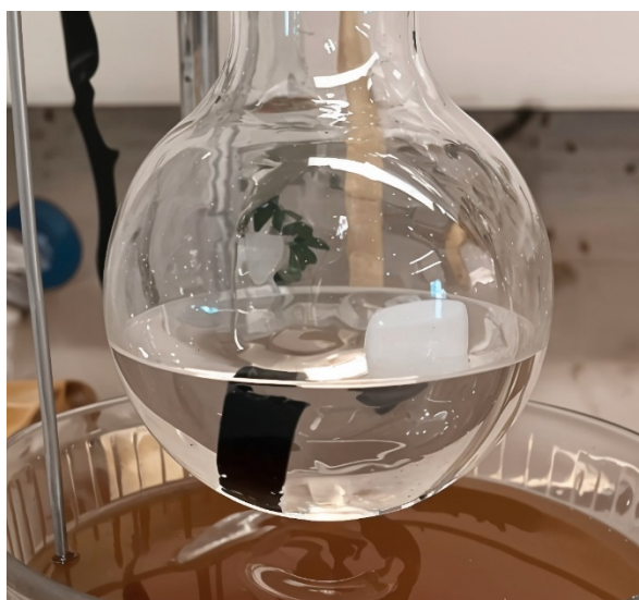
Figure S23. Extraction of particulate lignin-based hydrogel with tetrahydrofuran at 70 °C after 48 hours. The clear solution confirms the absence of LNP leaching, and, along with the gel content calculation (>98%), indicates the complete integration of LNPs within the hydrogel matrix.
