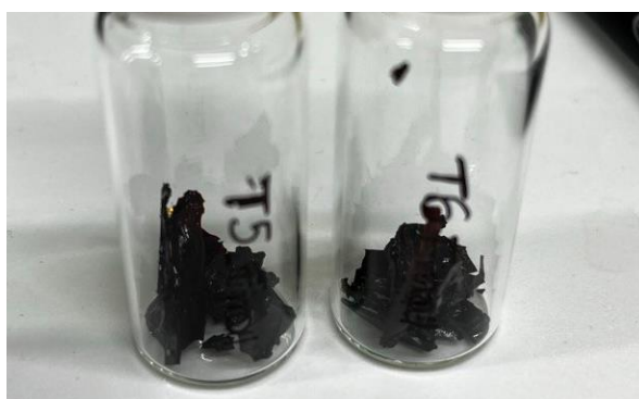
Fig. S25 – Picture of a first batch of thermosets without erythritol bis-cyclic carbonate as third component, with CC:NH 2 ratio of 1:1 (left) and 1:1.5 (right). The material was brittle and broke during IR measurements.
