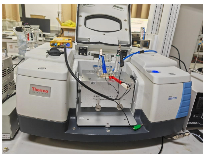
Figure S30. Diagram of electrochemical in situ ATR-IR equipment.
